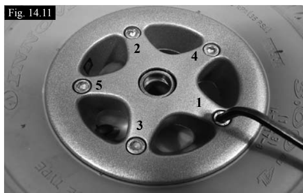
In the case of pneumatic tyres, let the air out of the tyre. Undo the 5 studs in the sequence shown. Refit and tighten to a torque of 15-20Nm. (Fig.14.11).
