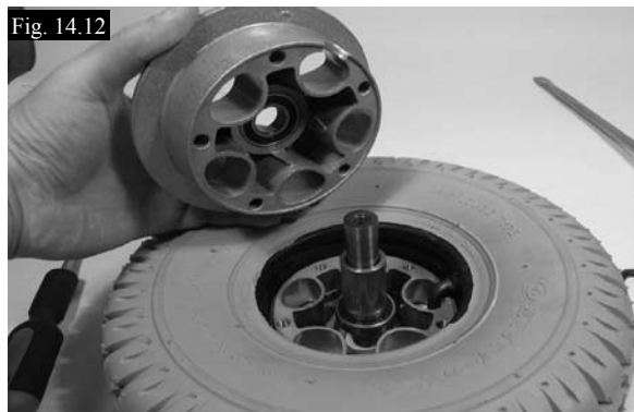
Lift the hubs out, (Fig.14.12).
