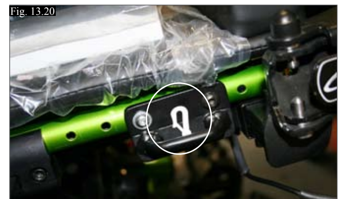
(Fig.13.20) Front tie down Powered Options.
