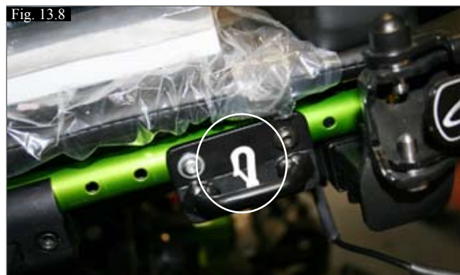
(Fig.13.8) Powered Option front tie down.
