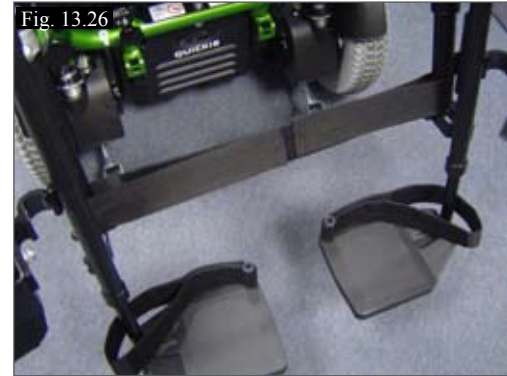
(Fig.13.26) Fit the strap around the Actuator shaft.
