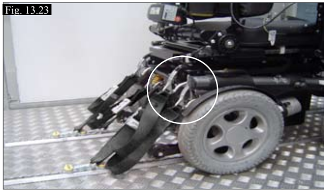
(Fig.13.23) Rear tie down positions. Use 4 straps.
