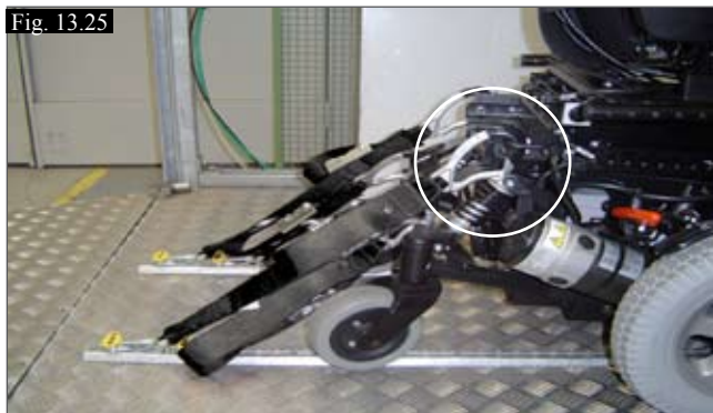
(Fig.13.25) Rear tie down positions. Use 4 straps.
