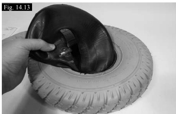
Gently feed the tube out of the tyre, (Fig.14.13).
