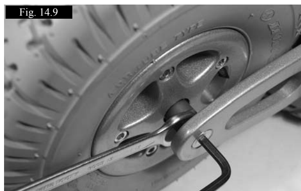
Use a 5.0mm hex key & 13.0mm open spanner to remove the axle studs, (Fig.14.9).
