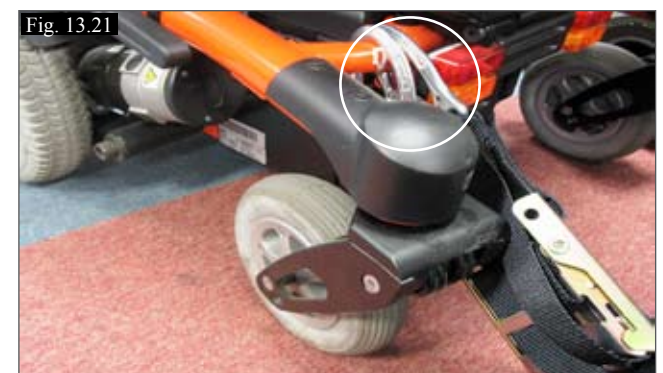
(Fig.13.21) Rear tie down position. Use 4 straps.
