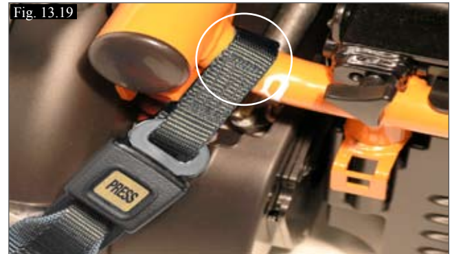
(Fig.13.19) Front tie down position, (no powered options).
