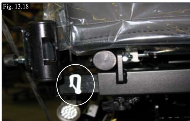
(Fig.13.18) Width Adjustable Hangers tie down.
