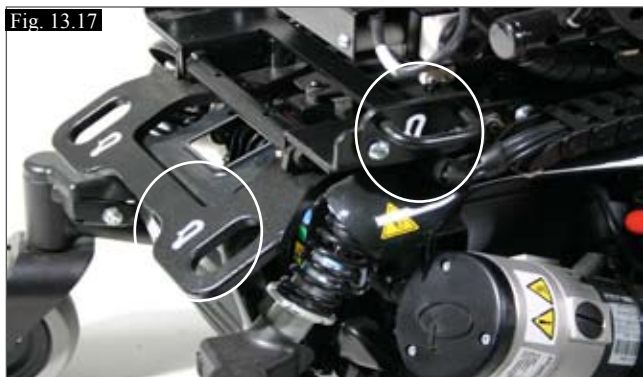
(Fig.13.17) Rear tie down for all options, (1 strap on each).
