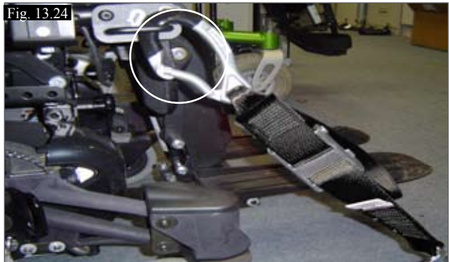
(Fig.13.24) Front tie down position, powered options. (Use bracket on frame for no powered options, Fig. 13.15)
