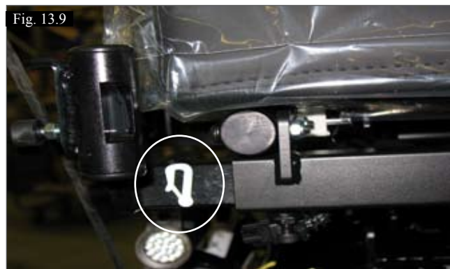
(Fig.13.9) Width Adjustable Hangers tie down.
