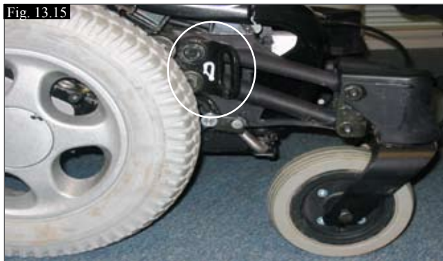
(Fig.13.15) No Powered Options, (no lift or tilt), front tie down.
