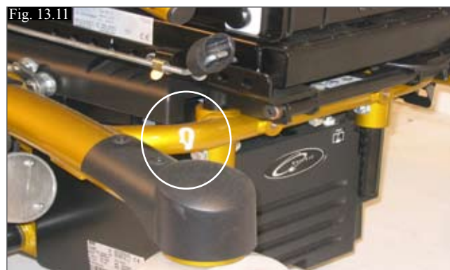
(Fig.13.11) No Powered Options, (no lift or tilt), front tie down.
