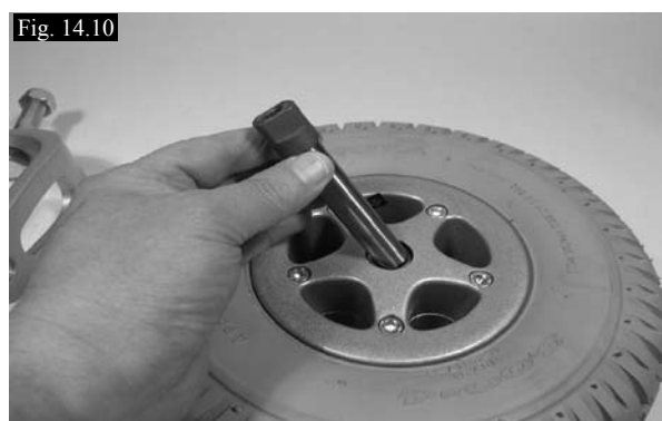
Remove the centre spindle, (Fig.14.10).
