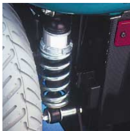
Full independent adjustable rear wheel suspension
