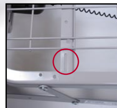
Slots in frame ensure proper rail placement
